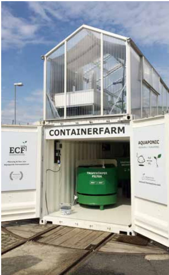
Prototype of container farm tested by Efficient City Farming (ECF) with aquaculture in container and hydroponics in greenhouse. Photo: ECF Farmsystems Berlin
