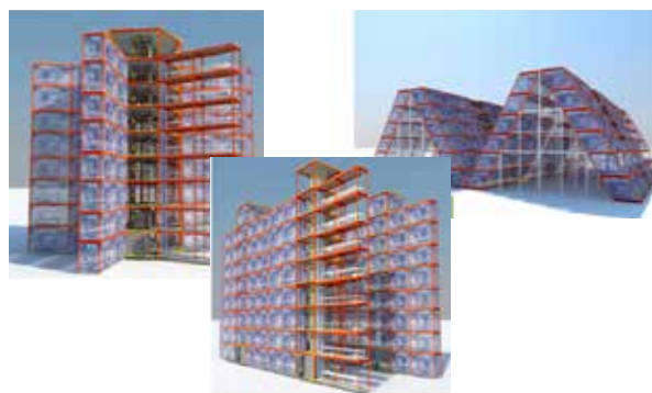
Geometric configurations using the basic modular “scaffold” structures for various farms: for the Cylinder Minimally Structured & Modular Vertical Farm (cMSM-VF) (left), Linear Minimally Structured & Modular Vertical Farm (lMSM-VF) (Middle) and Pyramidal Minimally Structured & Modular Vertical Farm (pMSM-VF) (Right).
