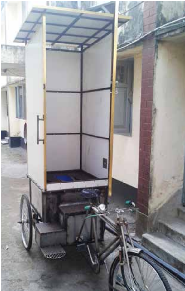
Mobile toilet designed by Practical Action, Bangladesh (article on page 77). Photo: René van Veenhuizen
